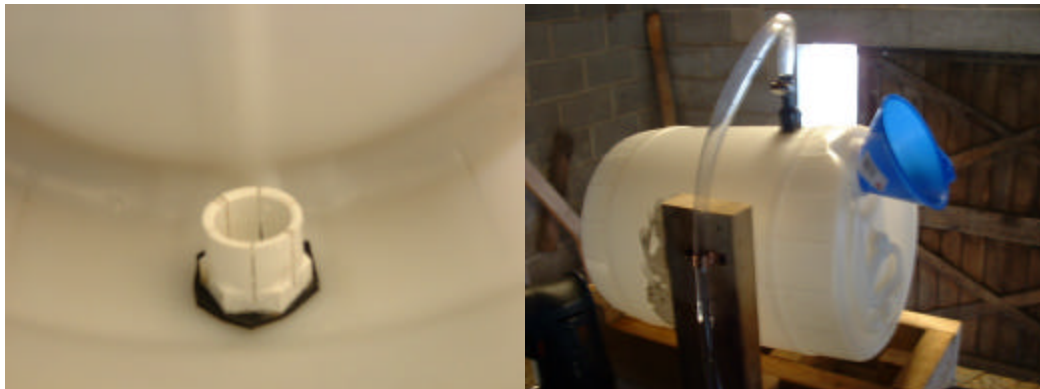
Figure 3.1.7 Methoxide Mixing Tank fitting as seen from inside the tank
